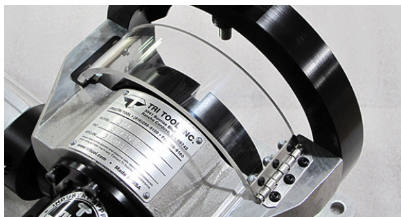
New for 2016 is the integral, clear chip guard designed to provide increased operator safety.
