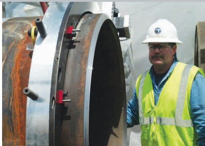
The high performance, second generation RBL-G2 brings improved speed and safety over the field proven RBL series of split frame lathes.
