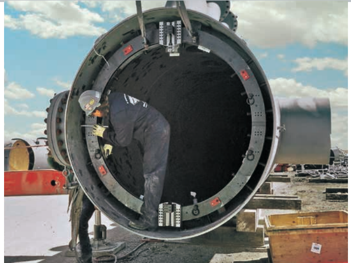
This 600 Series Clamshell is being used with the mounting screws and tool modules turned to cut from the inside out. Tri Tool's Services can assist you with custom and innovative equipment solutions for all your special machining and code welding requirements.
