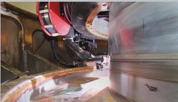
A Tri Tool DualARC® Weld Head is shown mounted to a custom SB Clamshell lathe performing a fill-in weld on a shaft the SB has previously machined.
