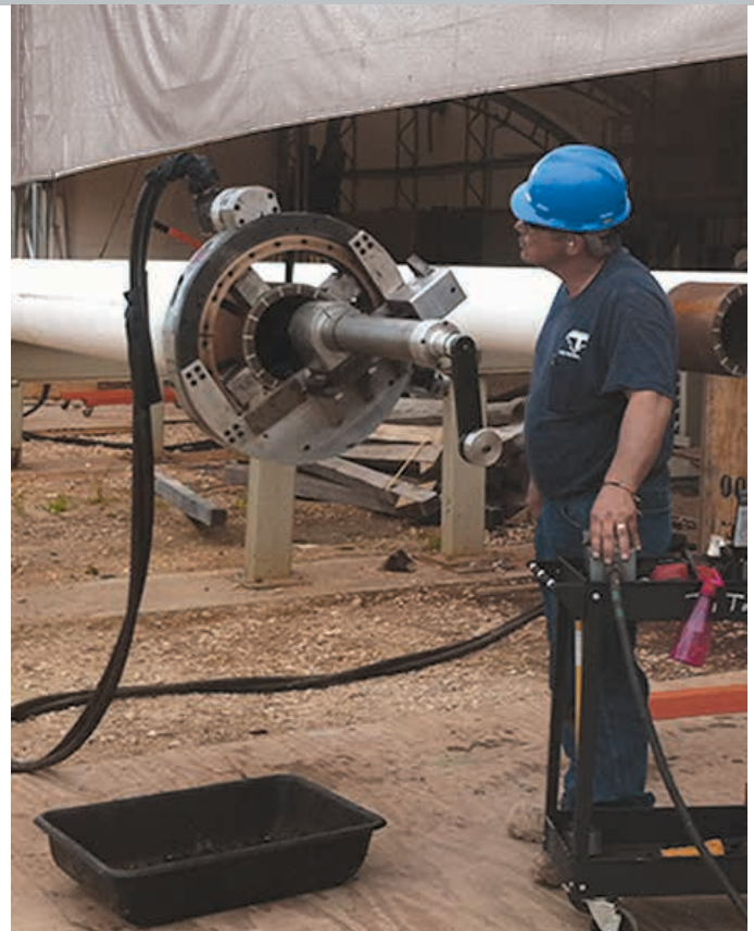
A 600 Series SB Clamshell performing a deep counterbore, critical to a pipe end-matching operation on an Oil and Gas Pipeline project.
