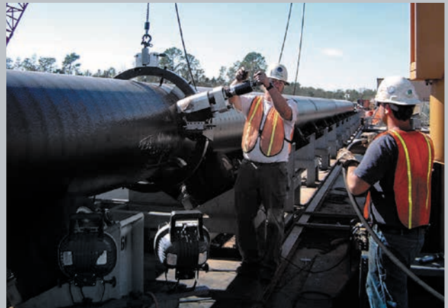
This Clamshell lathe has been configured to perform precision, in-line weld-profiling to strengthen weld joints for offshore platform tendon legs.
