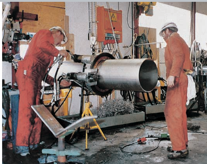
While most often used in a portable role, clamshells are extremely effective in fabrication shops where high volume, precise severs, bevels and end preps are needed. The above Clamshell is shown performing a simultaneous sever/bevel operation on titanium pipe.
