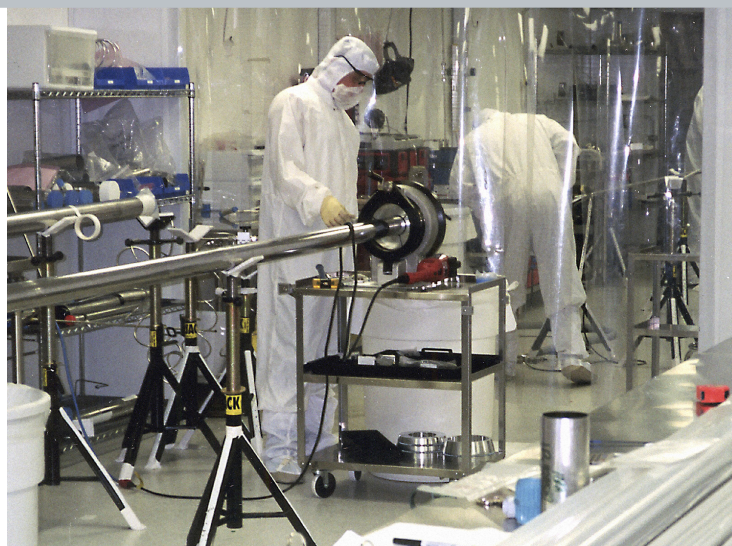
A Model 576AC being used to sever high-purity stainless tube in a clean room fabrication area. The ability to perform precision severs while protecting the tube's electro-polished ID makes the 500 Series the perfect companion to autogenous orbital welding operations.
