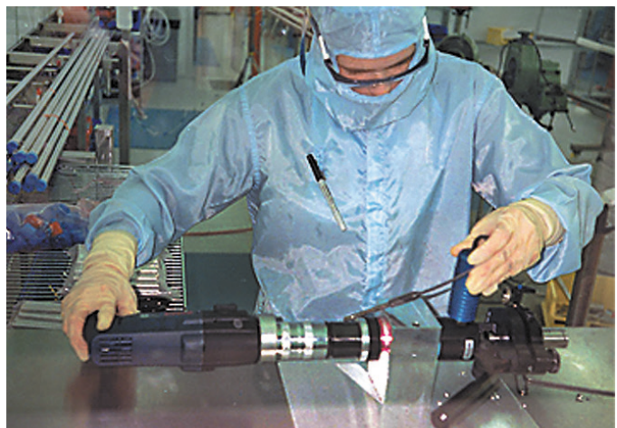
This custom engineered Model 301 has a heavy-duty motor and baseplate, a Quick-lock clamping system and a gear reduction unit to limit the tool bit rotational speed to deal with difficult alloys.
