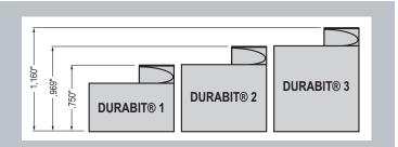
Premium DURABITs are "free cutting" (the edge stays under the chip) and extremely long lasting. Tool bits, designed for use with Tri Tool's 300 Series squaring equipment are made in three different lengths so that their entire cutting range is possible when using different saddle sets such as Short Perch saddles. Tri Tool will assist you in determining exactly the best bits for your specific requirements.
