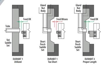
Squaring machines provide a short amount of precision bit travel. When using short perch saddles, a longer bit length is required to reach the microfitting stub.
