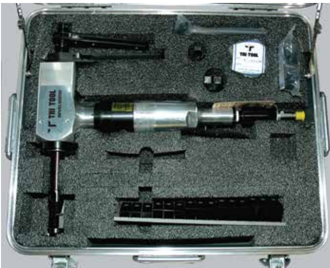
The BOILERMASTER® is a Model 204B with a ratchet feed, the perfect solution for boiler work.
