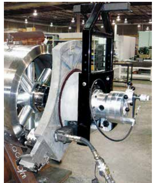
A Model 236B BEVELMASTER has been modified to include an auto-feed mechanism.
