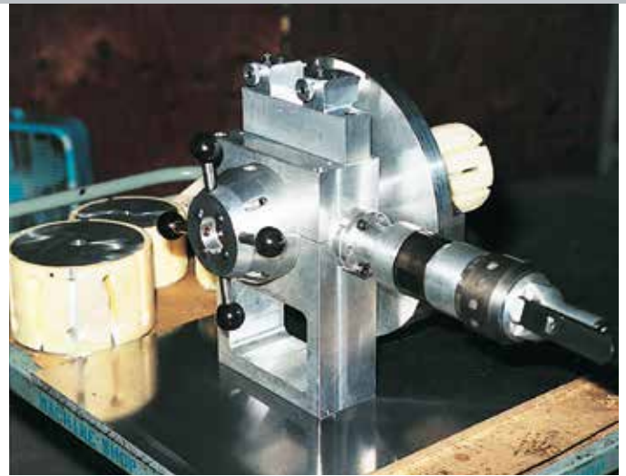
A BEVELMASTER set-up for high volume thin wall tubing production with several optional sleeve mandrels, bench stand, and dual trippers for rapid severing.
