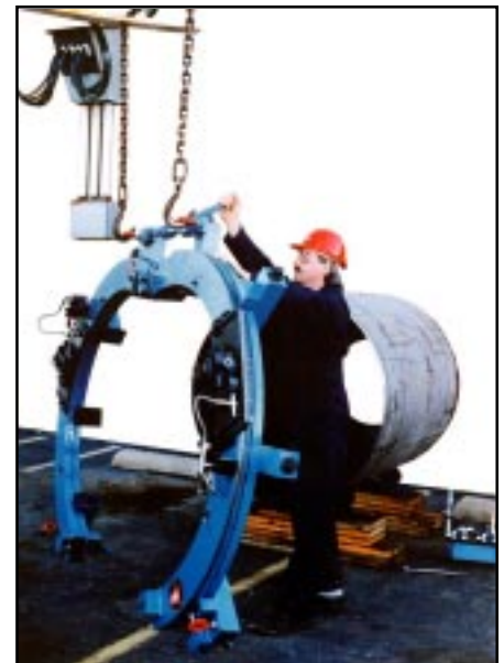
Frame assembly rachets open quickly
