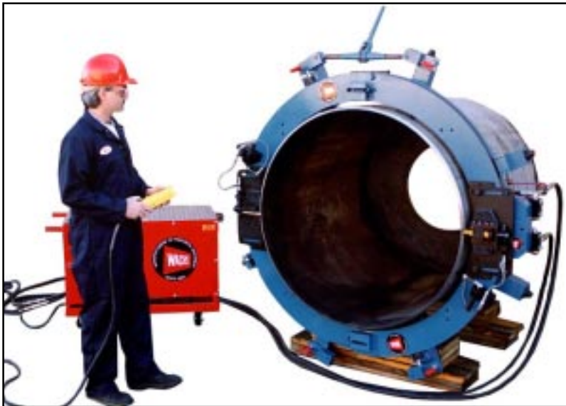
Operate using the optional remote pendant control
