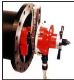
Convert from beveler to flange facer in minutes with the Flange Facing Module for raised and flat face flanges from 3.75" (95.2mm) I.D. through 24" (609.6 mm) O.D.
