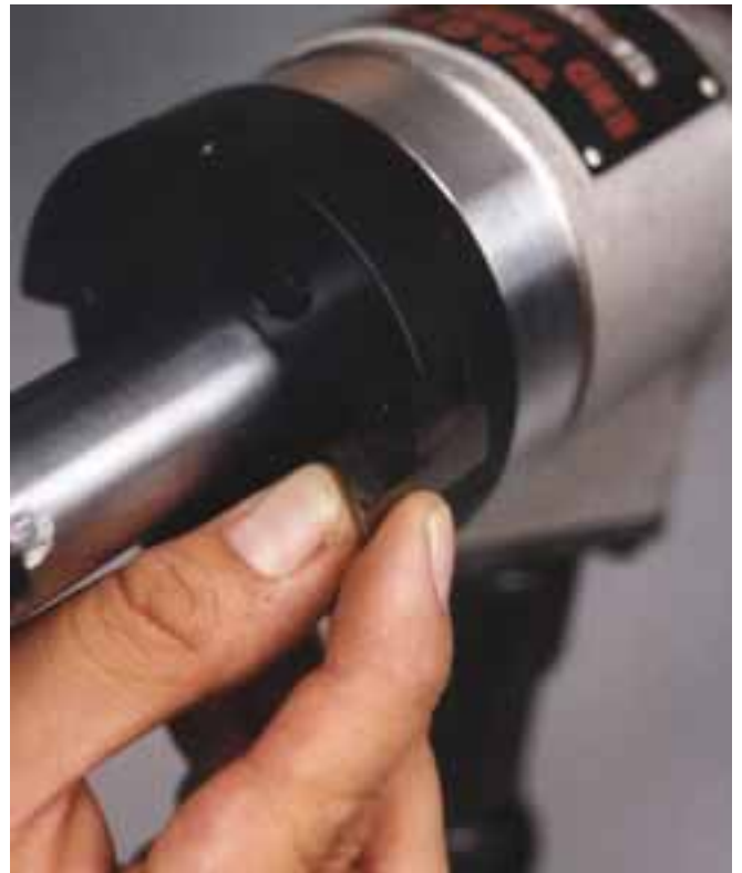
The new wedge style rotating head is a direct replacement for the old SBD rotating head and is secured in the same fashion.
