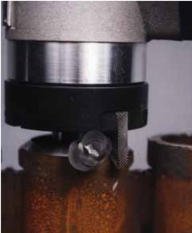
The new 70-700-00 beveling tool provides a smooth clean prep.
