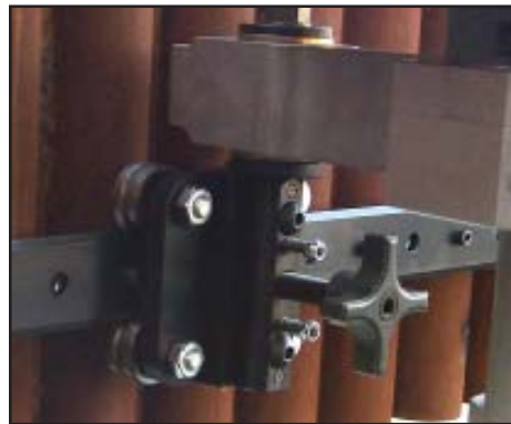
Panel Pro "Easy guide" slide assembly
