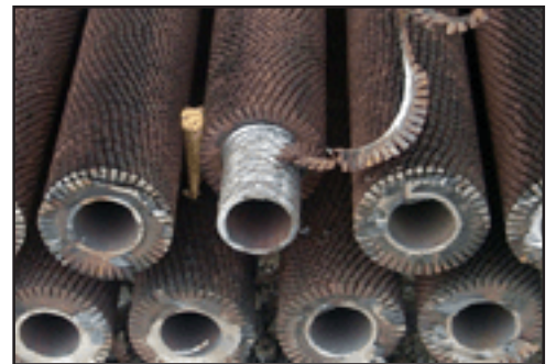
Fintube machining peel back
