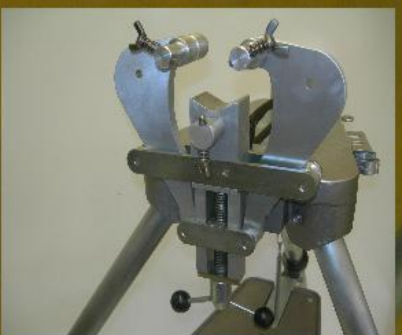
PIPE FITT UP CLAMP
