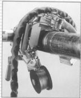
Pivoting Spool Mount – Unique design maintains tension on wire, prevents bending (not required on Model 433)
